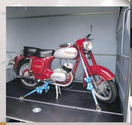
**Using Taki-Fixing system** you can lash different kind of goods safe, fast and easy.
